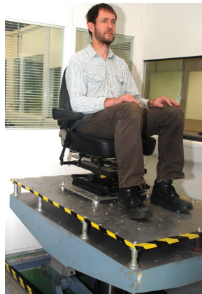
Laboratory testing of the vibration transmissibility of a suspension seat
